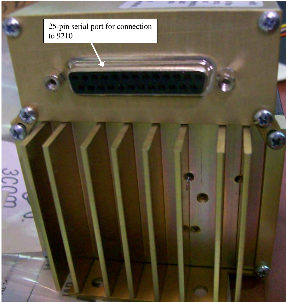
Figure 2: Back of DL3282 Modem showing 25-pin Serial Port
